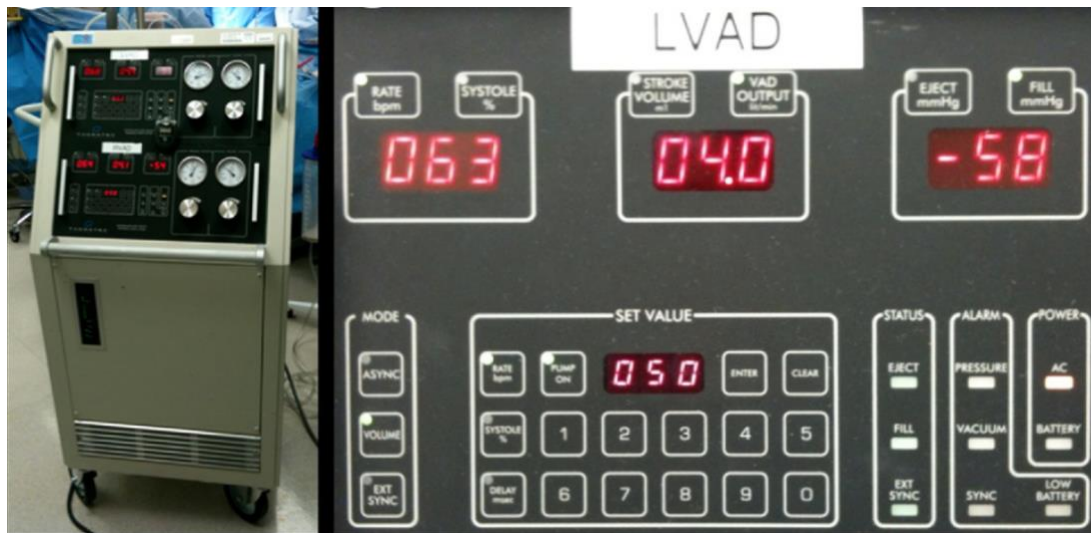
Photo of an early generation LVAD (left) and its control panel (right).
